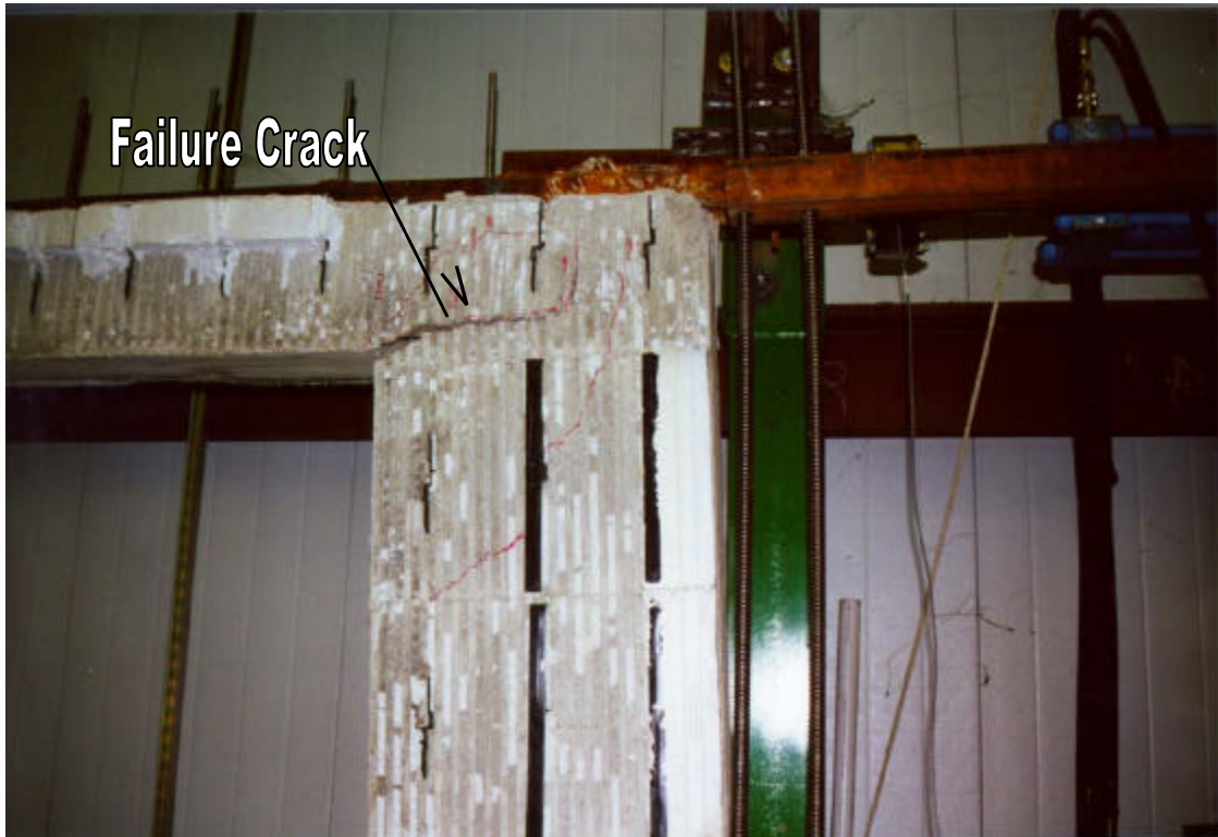
Figure 5 Failure Mechanism of Flat No. 3 Wall Specimen
