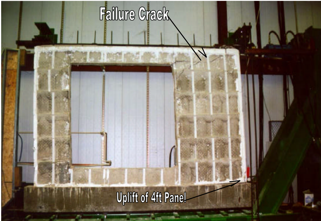
Figure 9 Failure Mechanism of Waffle No. 2 Wall Specimen
