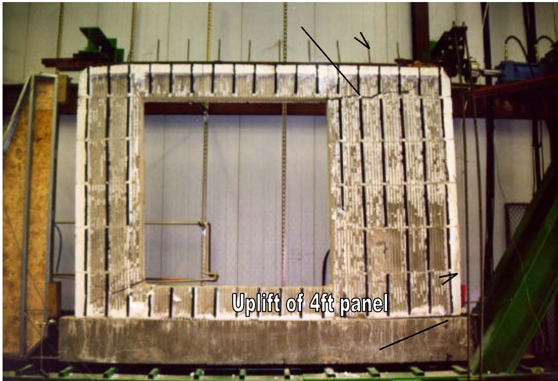
Figure 4 Failure Mechanism of Flat No. 2 Wall Specimen
